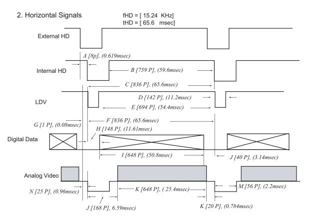
TM-6710/6710CL High-Speed Progressive Scanning CCD Camera **PULNIX**®
